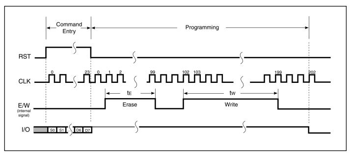
Figure 8. Programming Erase and Write
