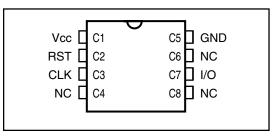
Figure 2. Pin Configuration
