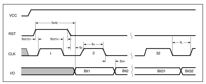
Figure 3. Reset and Answer to Reset Timing Diagram
